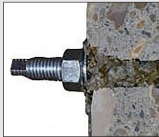
Anchor rods in solid concrete
